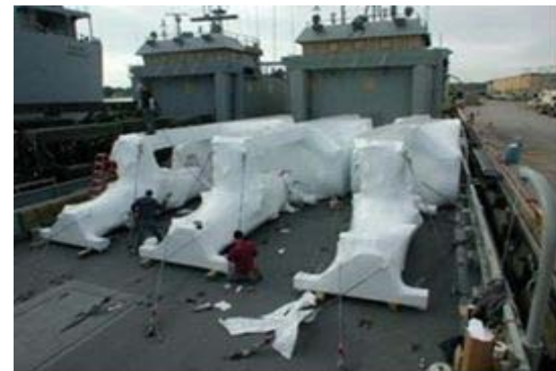
Effective shrinkwrap allowing safe deck top shipping
