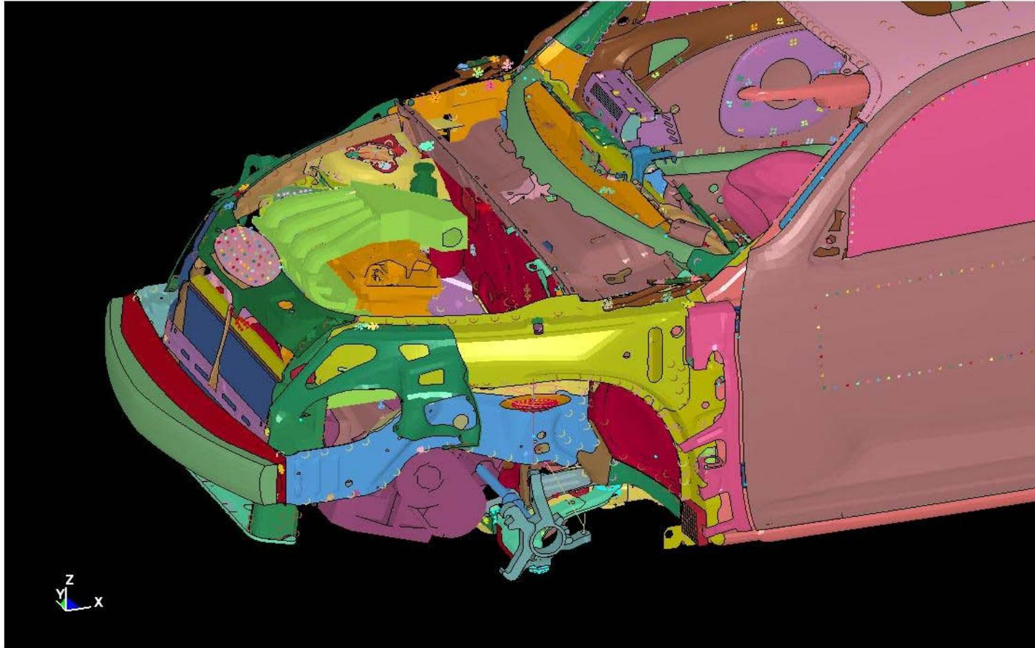
Manufacturing: Thermo-mechanical Models of the manufacturing process also save time and money - a goal is to model the manufacturing of the part and insert it, residual stresses and all, into the assembled automobile model\*
