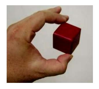
Cubes are gun launched in any axial orientation any number of times. Each sample is individually tested.
