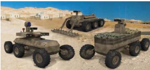
The FCS MULE's Three Variants: Assault, Countermine, and Transport
