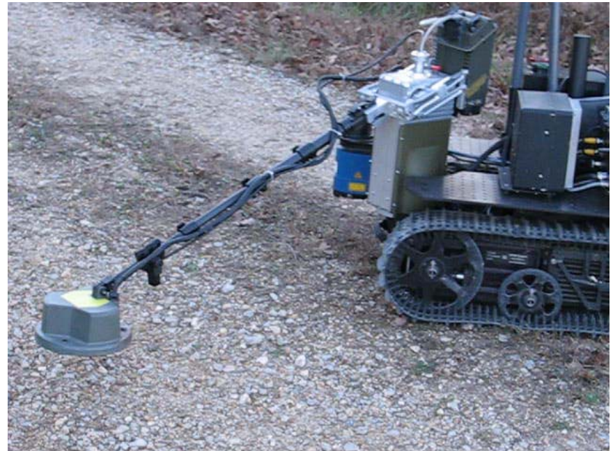
Prototype UGV with Mine Detector and Mine and Lane Marking System
