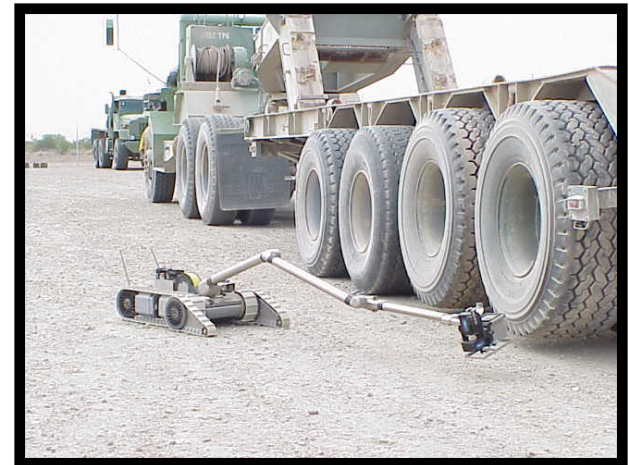
Packbot Version of MTRS Fido XT Sensor Payload
