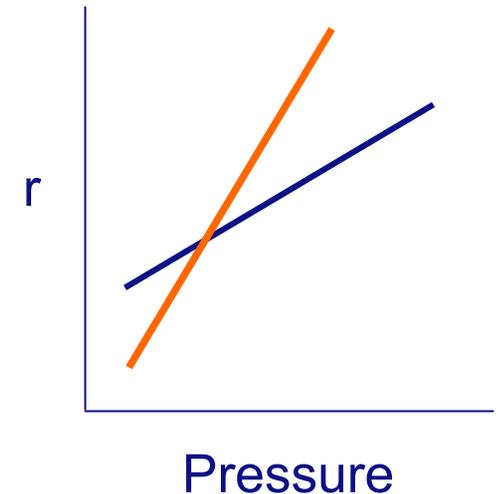
→ ignition phase LOVA's: low pressure → low burning rate → **lengthy and variable ignition delays**
