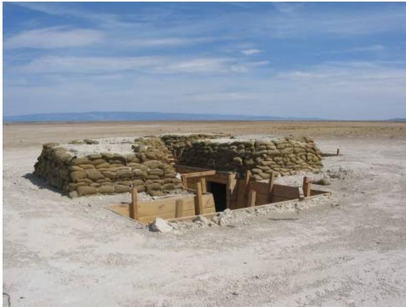
Earth & Timber Bunker Pre-Test Setup
