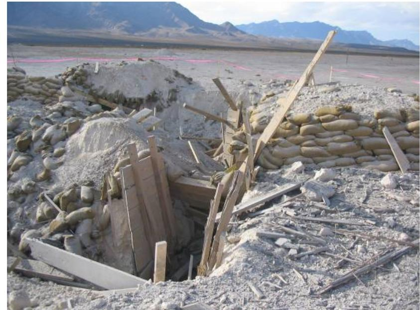
Earth & Timber Bunker Post-Test
