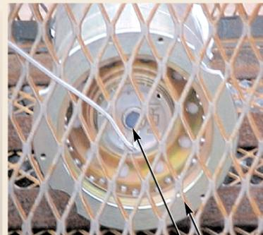
Thermocouple (flame temp)
