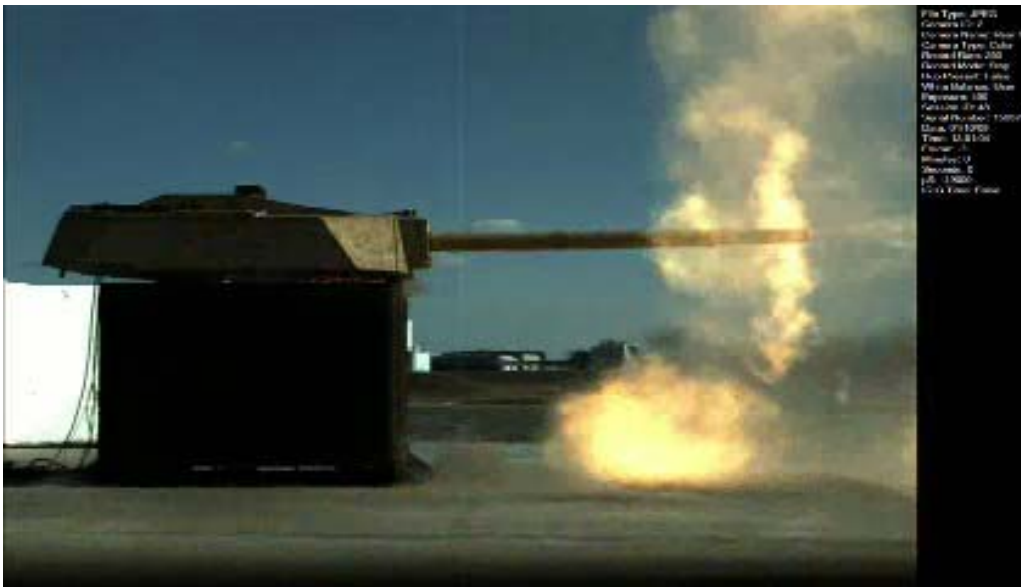
120 MM XM360 Firing off XM1202 Mounted Combat System Turret – Aberdeen Test Center – January 2009.
