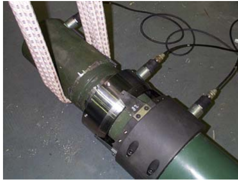
Natural Frequency Response Testing of 120 MM Tube
