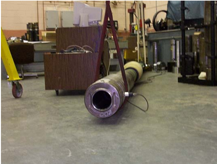
Natural Frequency Response Testing of 120 MM Tube
