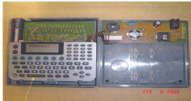
Small organizer fits neatly inside of POS terminal, skimmer and battery pack behind organizer.
