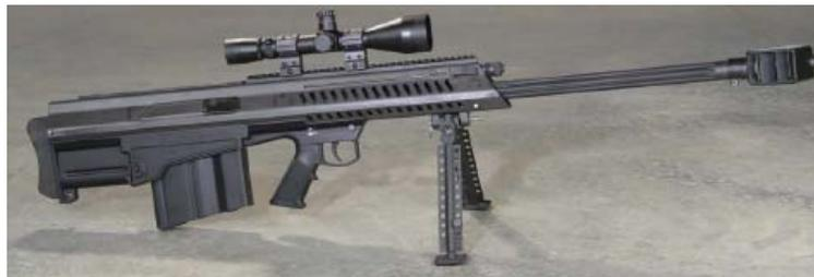
XM500 AMR .50 Caliber 26 lbs (Gas Op. Semi) – Lighter / Shorter than M107 at 46 inches long
