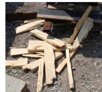
Pine Boards – 6 inches thick (4 boards) 18 gage steel W1& W2 were penetrated completely
