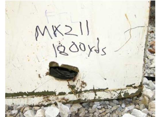
1800 yard MK 211 into target face and completely penetrated without activation
