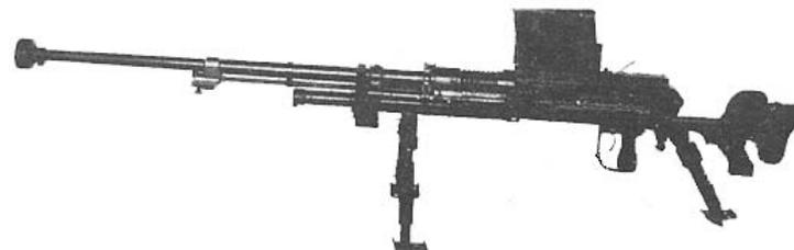
**Japanese Type 97 20X125mm @ 130-140 lbs rear monopod dug in for felt recoil reduction**
