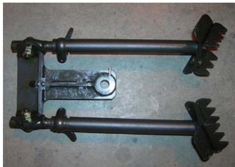
**NTW-20 bipod digs in and transfers a portion of recoil energy into the ground when prone. Adding a spiked rear monopod – forming a reversed tripod – could also help reduce felt recoil considerably.**
