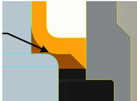
Contact should be farther out radially to eliminate annular depression
