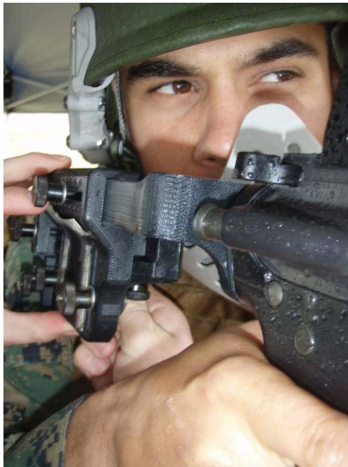
Test rig redesigned to accommodate lateral positioning 2cm closer to the face for offset sights
