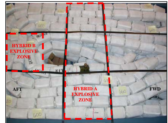
Typical View of MICLIC HYBRID SYSTEM A & B M58 shipping container.
