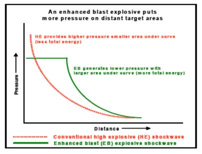
Fig. Comparison of conventional explosives and enhanced explosives.
