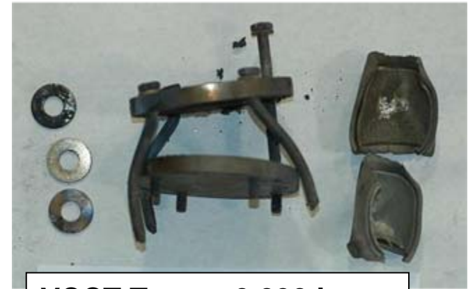
VCCT Test at 0.090 in. Wall Thickness
