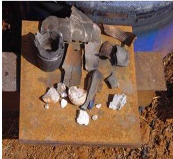
Figure 6: Liquid Fuel Fire for 76/62 mm HE ammunition test results
