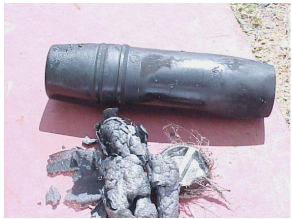
Figure 19: Liquid Fuel Fire test result for 76/62 mm filled shell with main charge NREV 9506 with no booster
