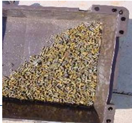
Figure 7: Liquid Fuel Fire for 76/62 mm SU PRAC ammunition test results
