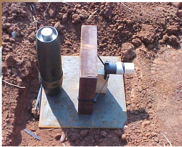
Figure 20: Shaped Charge Jet Impact set up and results: RXHR-5 main charge formulation
