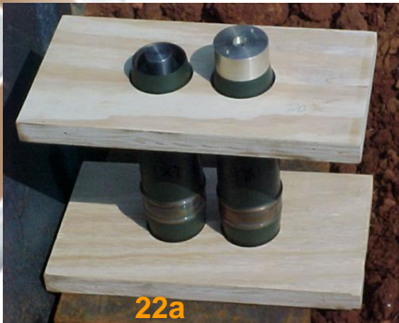
Figure 22: Test set up for Sympathetic Detonation with varying air gap for RXHR-5
