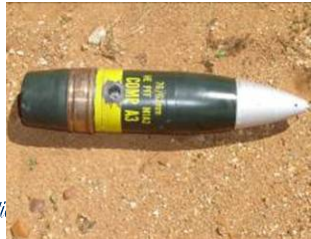
Figure 11: Bullet Impact test results for 76/62 mm HE and PFF through main charge
