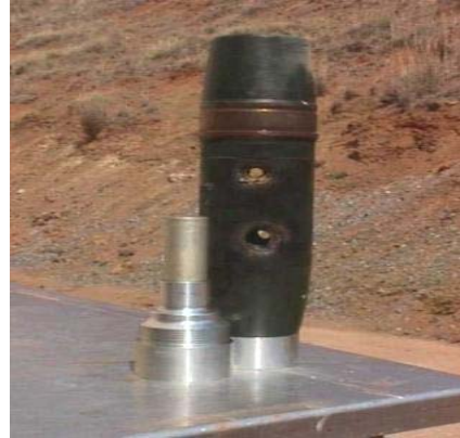
Figure 22: Test set up for Sympathetic Detonation with varying air gap for RXHR-5
