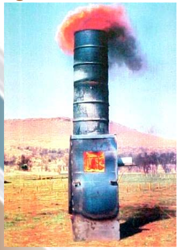
Figure 19: Liquid Fuel Fire test result for 76/62 mm filled shell with main charge NREV 9506 with no booster
