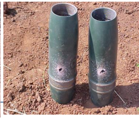
Figure 20: Shaped Charge Jet Impact set up and results: RXHR-5 main charge formulation
