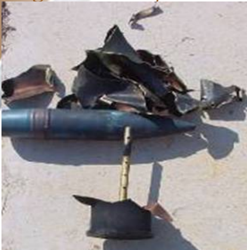
Figure 7: Liquid Fuel Fire for 76/62 mm SU PRAC ammunition test results
