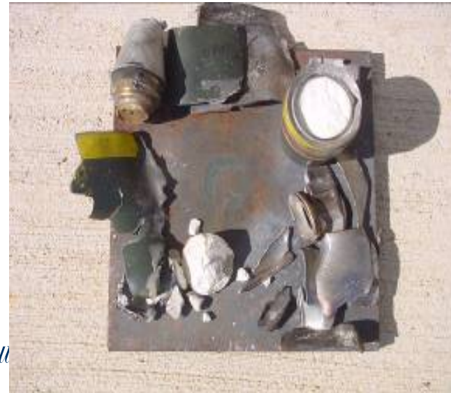
Figure 16: 76/62mm HE PFF Shaped Charge Jet results
