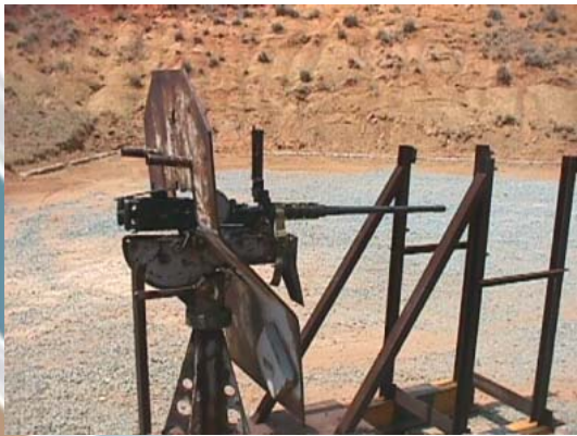
Figure 22: Test set up for Sympathetic Detonation with varying air gap for RXHR-5
