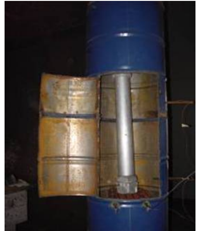
Figure 5: Liquid Fuel Fire for 76/62 mm ammunition test set-up
