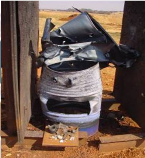
Figure 6: Liquid Fuel Fire for 76/62 mm HE ammunition test results
