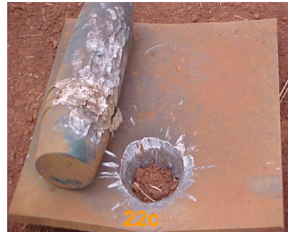
Figure 22: Test set up for Sympathetic Detonation with varying air gap for RXHR-5
