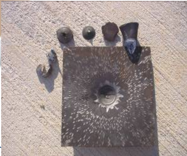
Figure 16: 76/62mm HE PFF Shaped Charge Jet results
