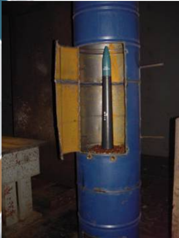
Figure 5: Liquid Fuel Fire for 76/62 mm ammunition test set-up
