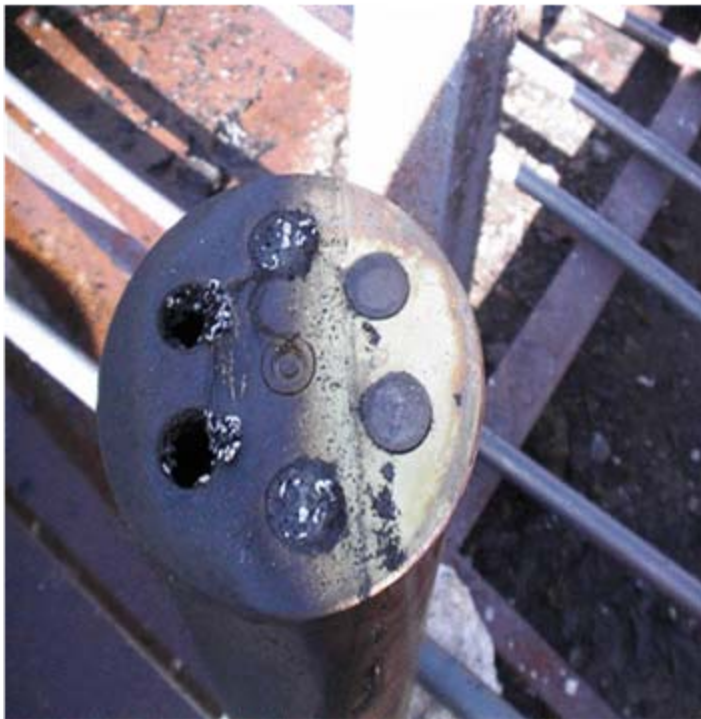
Formion plugs – carbonized instead of melting
