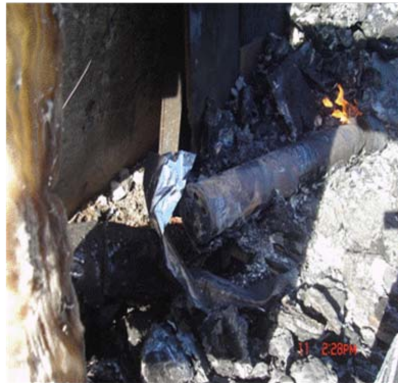
Cartridge case with holes at base
