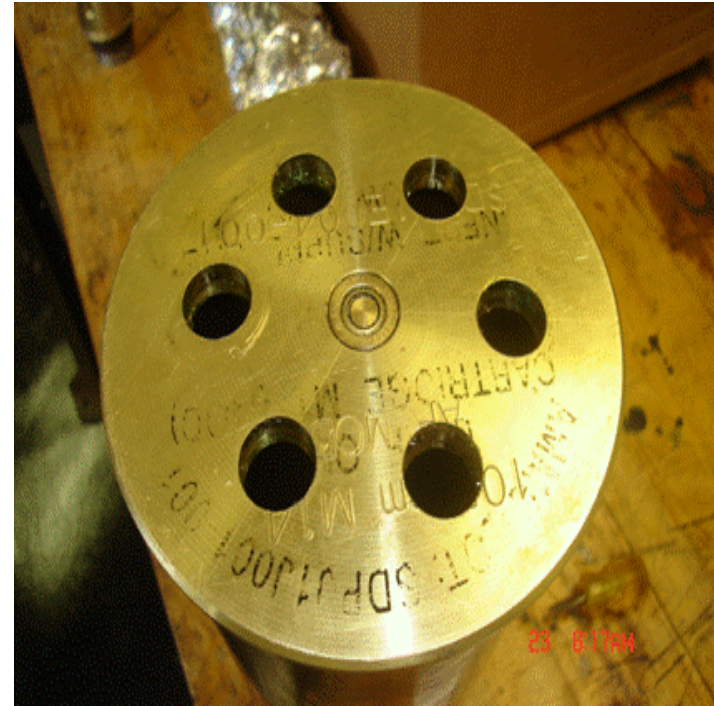
Cartridge case with 6 3/4" diameter holes at base
