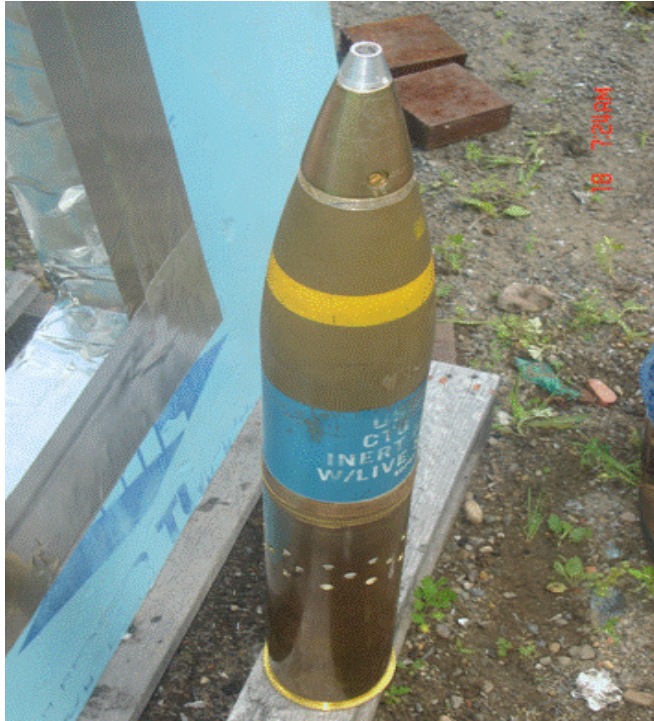
Cartridge Case with 30 3/8" diameter holes on forward end
