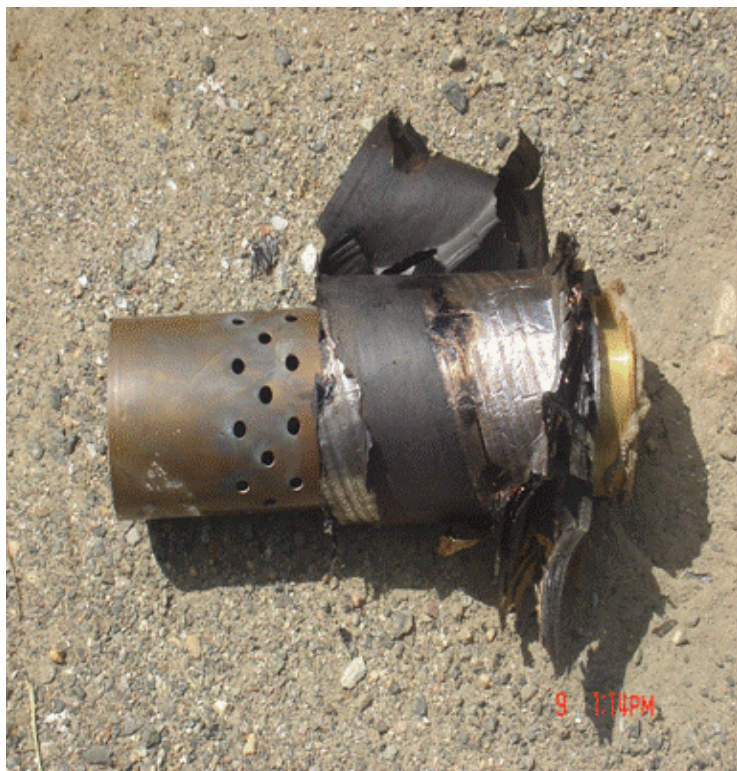
Cartridge case with holes at forward end
