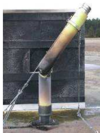
[ 27 ] Type IV ; BI PROPULSION NOT IN EVIDENCE SMALL FLOW OF GAS THROUGH NOZZLE
