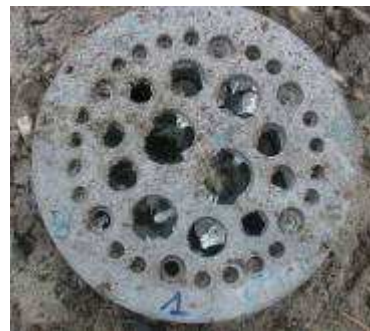
ALTERNATIVE BLAST PRESSURE MEASUREMENT METHOD “CHALARD BOX”
