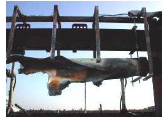
[51] Type V FH : Weakened Steel
