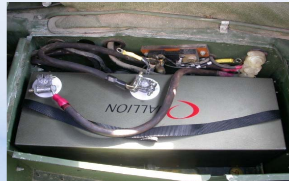
Quallion Drop-in Li-ion APU 24V, (78Ah, 98.8Ah, 156Ah), 52lb
