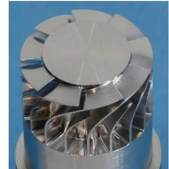
Turbine Rotor Fabrication Trial
