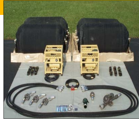
Medium System with (4) 155 Gal Bladders
