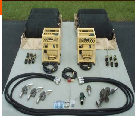
Small System with (6) 28 Gal Bladders
