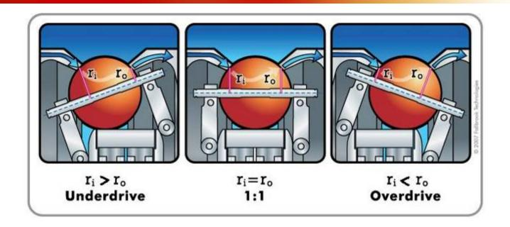
Speed ratio changes with contact radii ratio (r<sub>i</sub>/r<sub>o</sub>)
