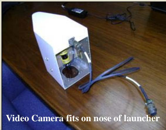
Video Camera fits on nose of launcher
