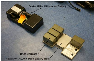
TALON BB-390/BB-2590 Battery Upgrade "6-PACK" -increase run time by 2 hrs
