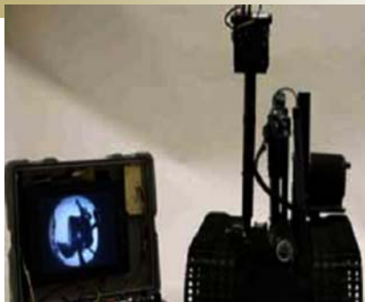
Wide Angle Remote View camera 180 degrees x 360 degrees. standard camera is: 54 degrees
