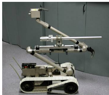
EOD Disrupter Integration onto MTRS Robots
