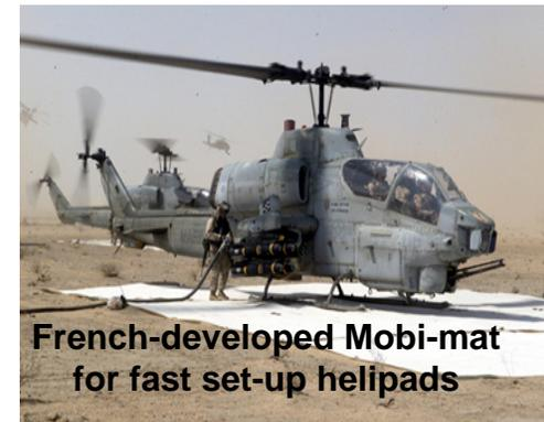
French-developed Mobl-mat for fast set-up helipads
