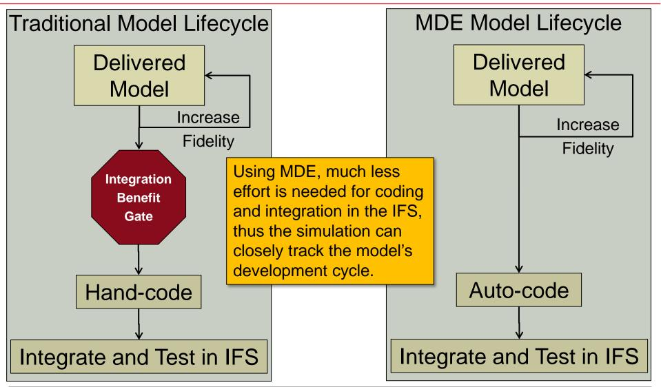
Autocoding can reduce cycle time for integrating updated models
