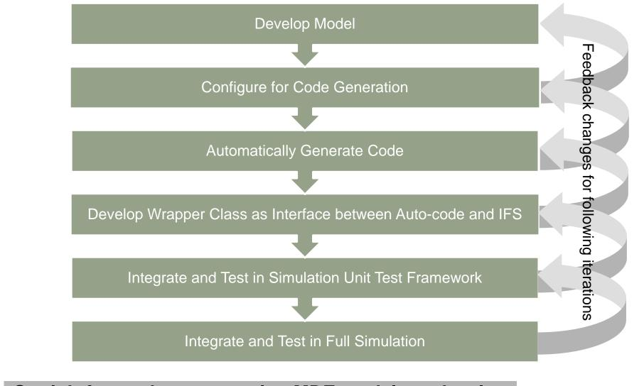
Straightforward process using MDE models to develop Functional Simulations
