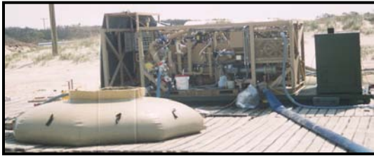
Tactical Water Purification System
