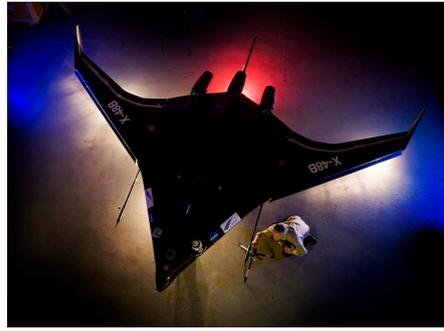
(scaled-down wind-tunnel model)
