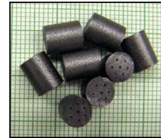
PAP-8386: Etherless Propellant for 120 mm Tank Training Rounds
