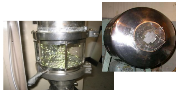
Sweetie Barrel & Fluidized Bed Coating of Propellants
