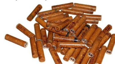
Caseless Cartridge bodies drying on mold cores
