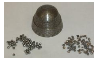
Sintered Tungsten Alloy Matrix
