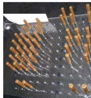
Caseless Cartridge bodies drying on mold cores
