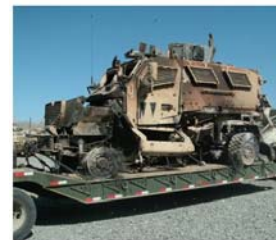
Exterior view of the MRAP after the fire.
