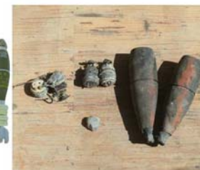
Shell bodies and separated M768 fuzes recovered from the vehicle after the fire.
