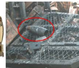
Interior view of the MRAP after the fire. An unexploded shell body from a M768 cartridge can be seen.
