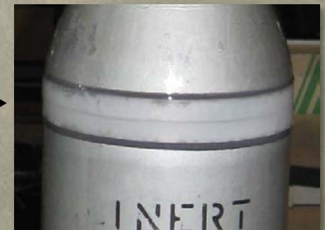
Polypropylene Band Edges Sealed with epoxy
