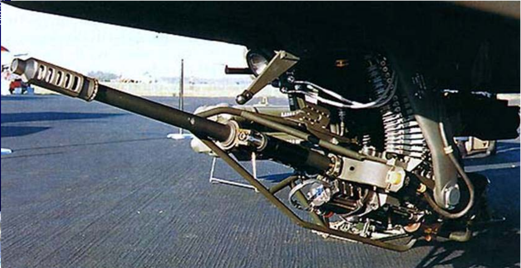
The Apache's 30 mm x 113 automatic M230 chain gun
