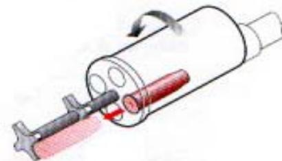
*Ejection of cartridge case*
