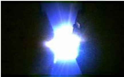
Vaporization of an IHDIV MEMS initiator
