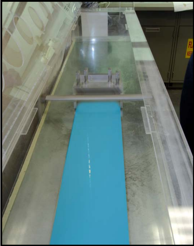
Lab-scale tape casting setup
