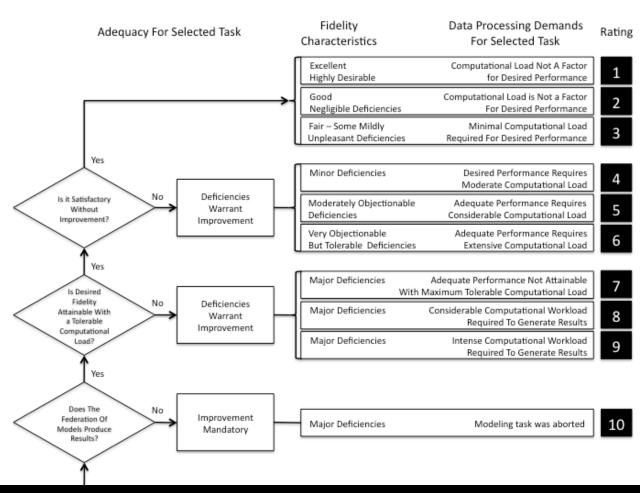
Based on the Cooper-Harper Handling Qualities Rating Scale
