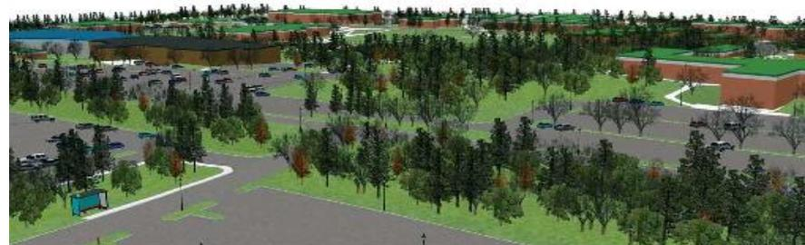
Completed database featuring elevation data, with overlaid imagery, and integrated GIS features compiled together into a synthetic environment.
