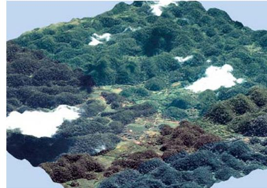
Application of Satellite Imagery onto the surface of the TIN
