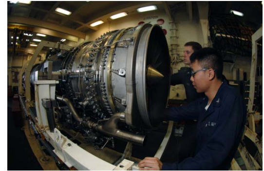
F414-GE-400 engine (U.S. Navy photo by Mass Communication Specialist Seaman Stephen W. Rowe/Released)
