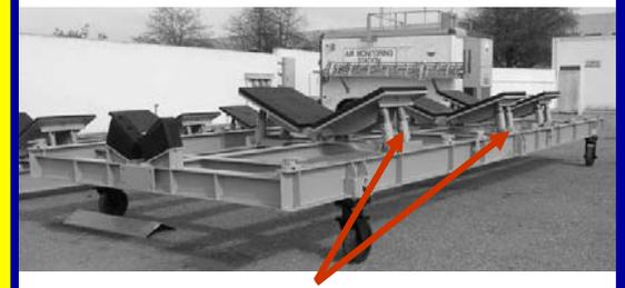
Adjustable support frames to interface with ASW USV (tri-hull) and MCM USV (monohull) and Navy Standard 11-m RHIB
