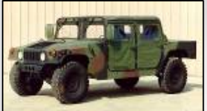
A0 Series (1984-93) 6.2L Diesel Engine 3 Spd Transmission 2,500 – 3,632 lb. Payload GVW: 7,700 lb.
