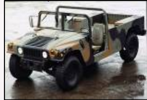
A2 Series (1994-Present) 6.5L Diesel Engine 4 Spd Electronic Trans 3,520 - 4,400 lb. Payload GVW: 10,300 lb.
