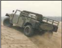
A1 Series (1991-95) Improved Driveline Improved Suspension 2,500 – 3,632 lb. Payload GVW: 10,000 lb.
