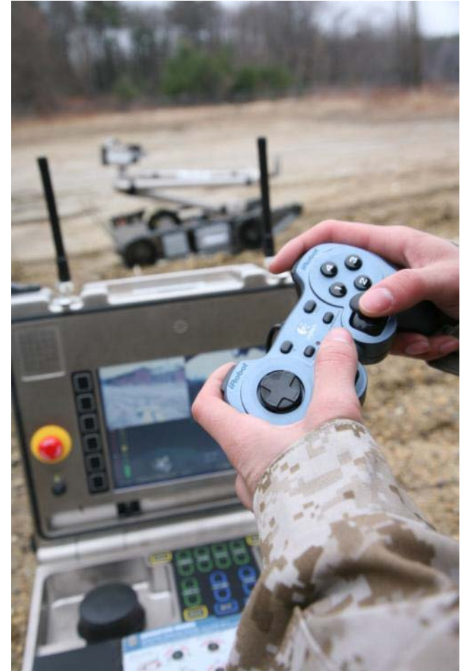
Today's controller and OCU.
