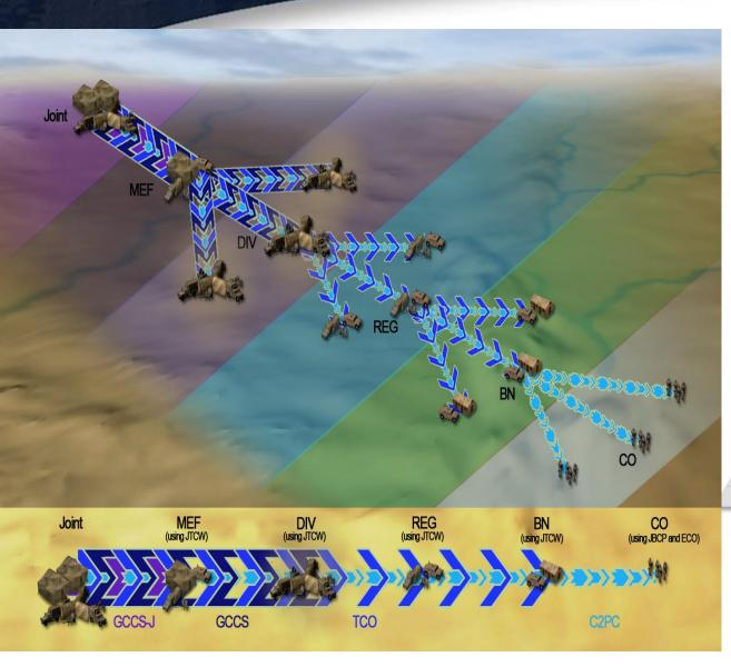
The COP is a two-way feed of information, coming down from the Joint level via GCCS-J, and coming up from the Company level via BFT/JBCP and ECO. At each level, the COP is viewed via C2PC.
