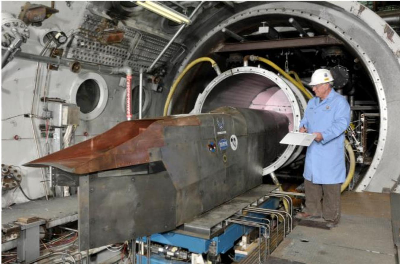
**AEDC APTU tests under FaCET of common turbo-ramjet/scramjet flowpath**
