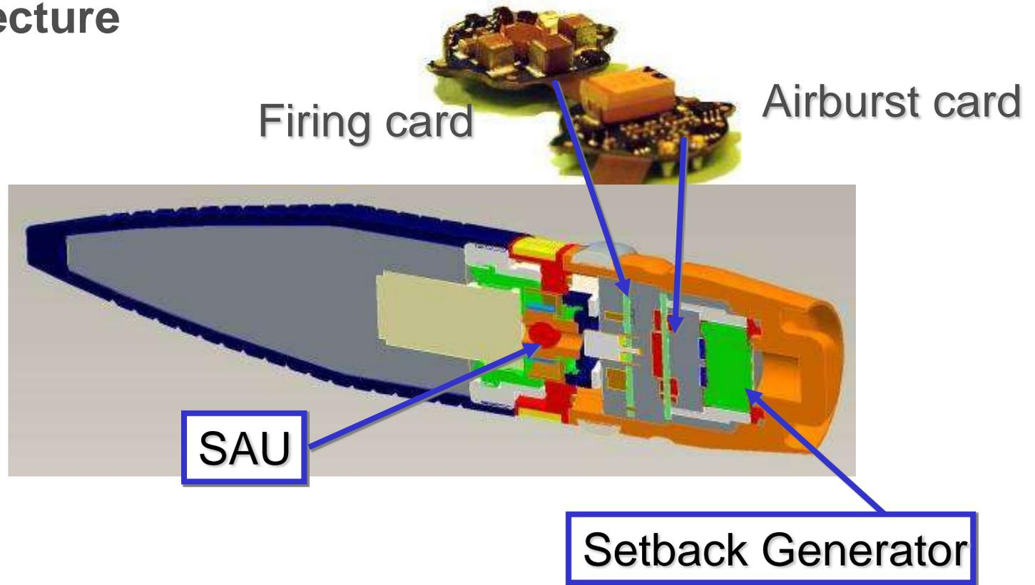
Electronics and SAU designs are deeply fitted into each other during engineering process.
