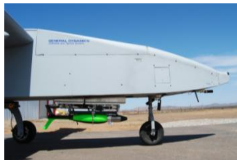
Tiger Shark UAV with 81mm Guided Air Drop Munition and GD-OTS Rack System
