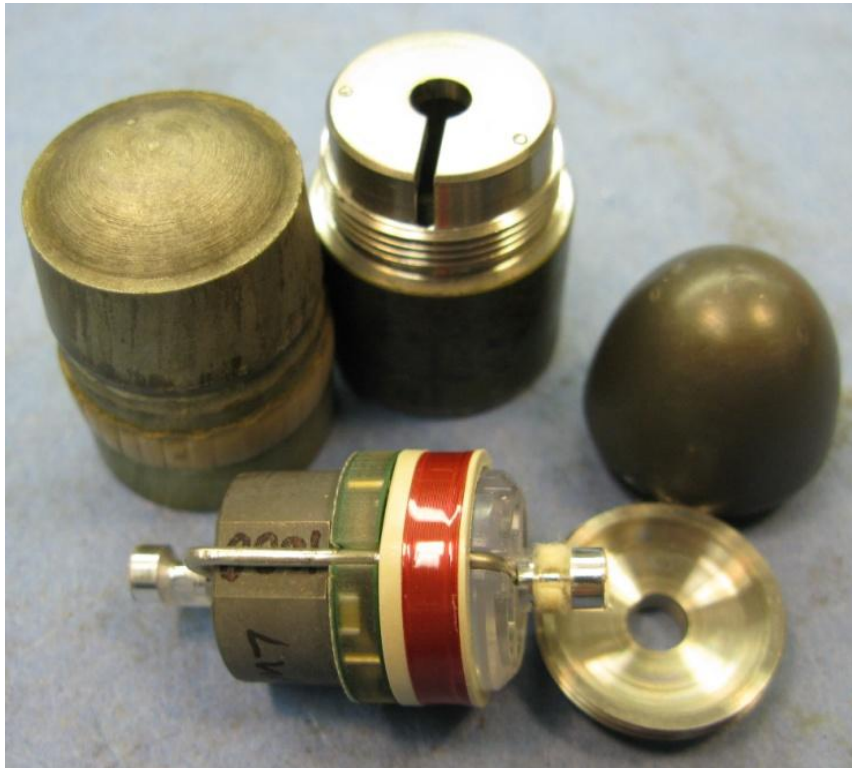
Mid-body Airburst Projectile Components
