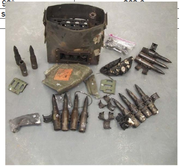
Post Test Results T/S 241-270 / Test 1 Slow Cook-Off Test
