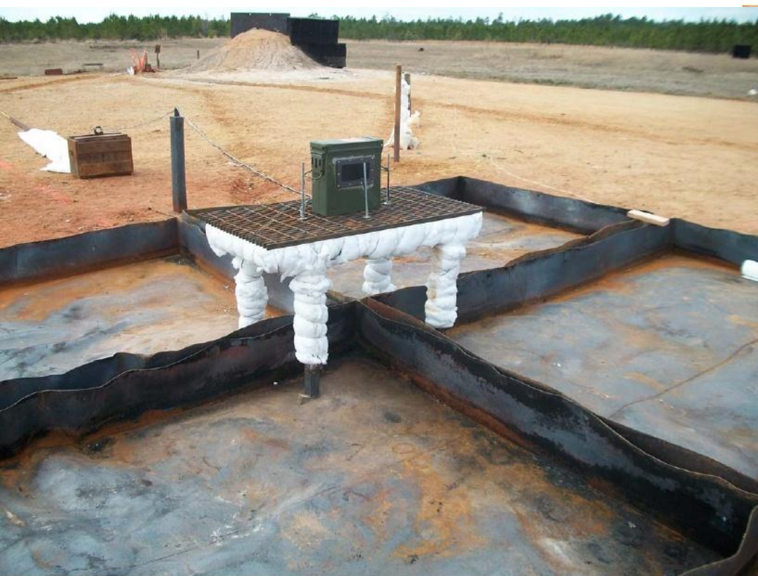
Test Setup T/S 121-150 / Test 1 Fast Cook-Off Test
