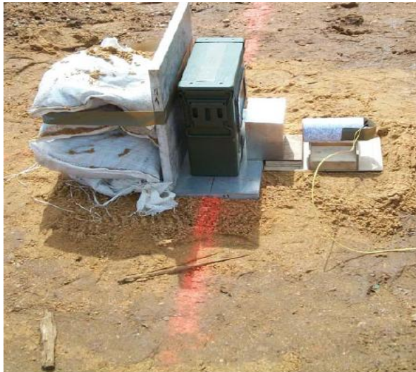
Test Setup T/S 1-30 / Test 1 Shaped Charge Jet Impact Test
