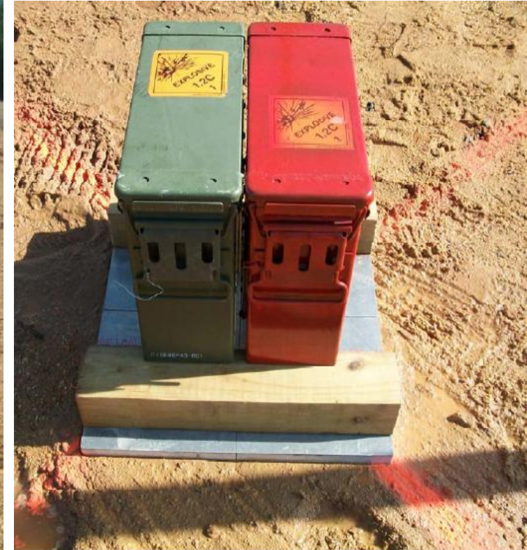
Test Setup T/S 61-120 Unconfined Sympathetic Detonation Test
