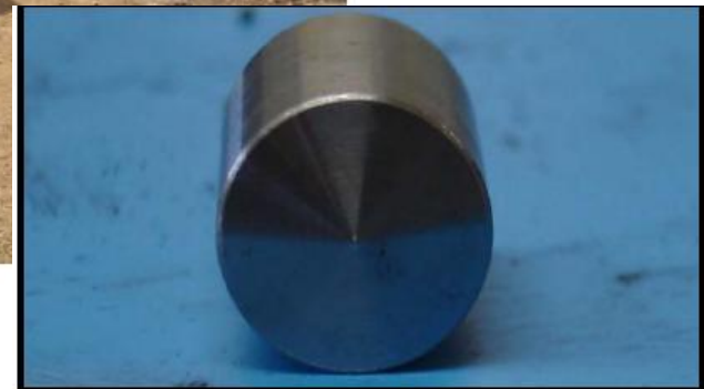
Figure 18 .50-in. mild steel conical army fragment
