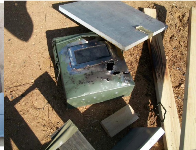
Post Test Results T/S 331-360 / Test 2 Bullet Impact Test
