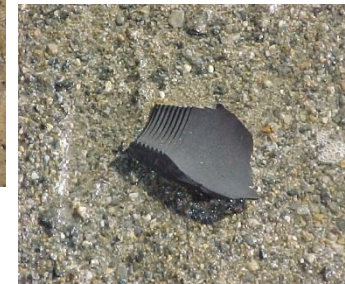
Projectile Body Fragments and Unconsumed COMP B Explosive (TYPE II Response)
