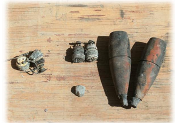
Burned-out 60mm M768 projectiles recovered from MRAP
