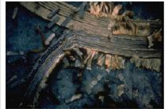
Figure 2-3. GIC Damage to Transformer During 1989 Geomagnetic Storm
